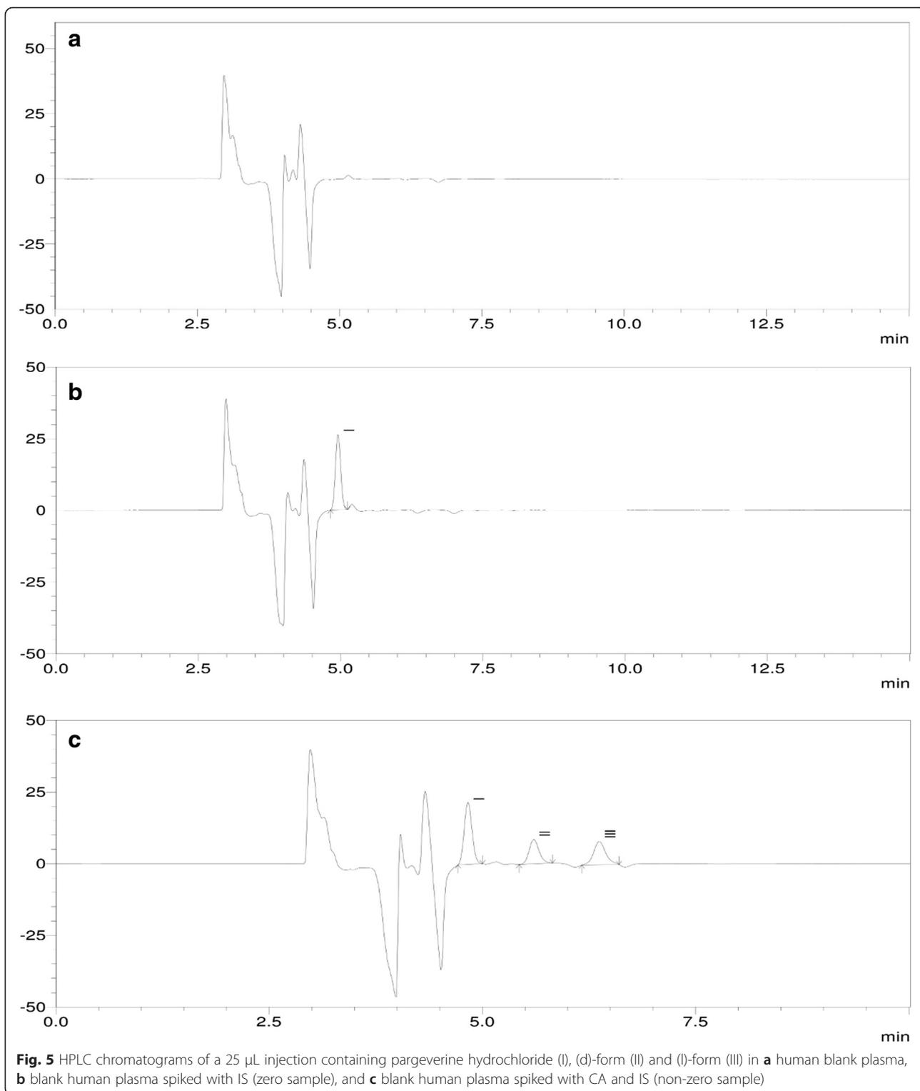
order to improve the peak shape. All chromatographic parameters were kept constant (flow rate, 0.8 mL/min, ambient column oven temperature; injection volume, 25  $\mu$ L; wavelength, 220 nm) except the % additive added.
