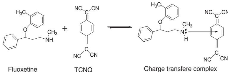
**Figure 5** The suggested reaction pathway between fluoxetine as representative example of the studied drugs with TCNQ.
